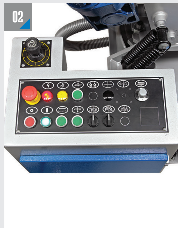
KUMANDA PANELİ CONTROL PANEL
